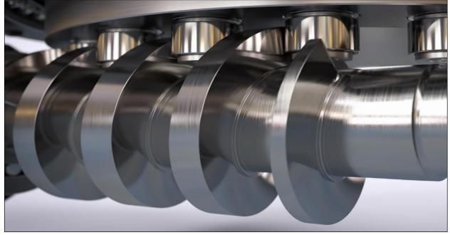
Optimized power transmission due to a minimum of three constantly engaged cam followers at any time – the reliable EXPERT-TÜNKERS Multi-Cam-Follower Principle!
