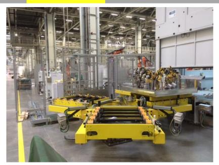
Puffer station for the toolings on the felx turntable
